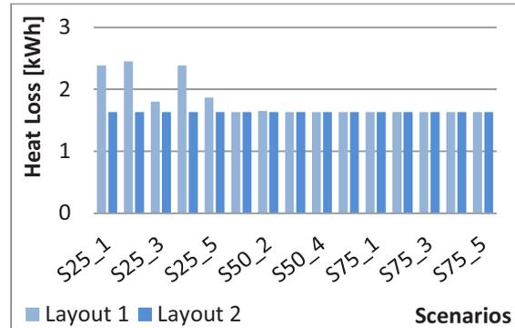
**Figure 11.** Overall heat loss observed at the return line in each scenario.
