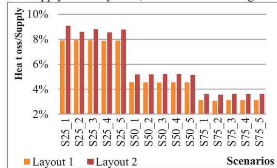
Figure 7. The overall heat loss from the DH network over the heat supplied from the heat source, observed through the whole time range
