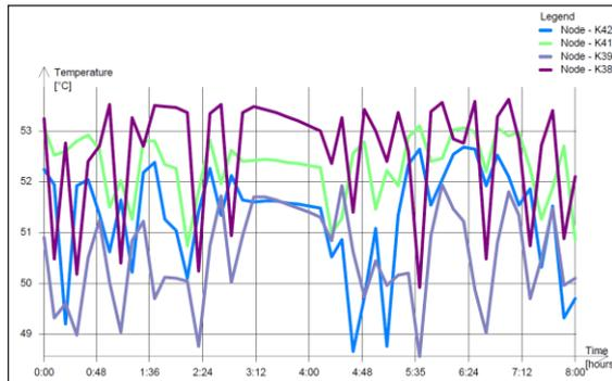
**Figure 9.** Supply temperatures observed at the end-nodes and predecessor nodes of them in the routes 3 and 4, in case of Layout 1
