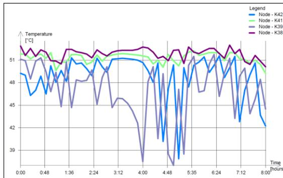
**Figure 10.** Supply temperatures observed at the end-nodes and predecessor nodes of them in the routes 3 and 4, in case of Layout 2
