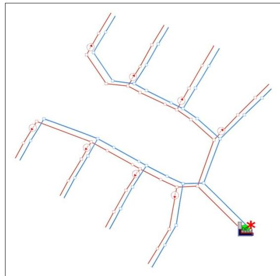
**Figure 2.** Branched type DH network with booster pumps, installed in the beginning section of each street
