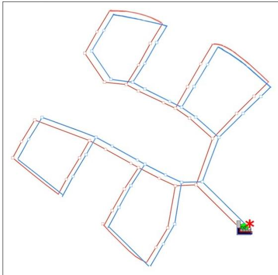
Figure 3. Looped type DH network
