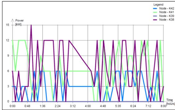
**Figure 8.** The time series of heat demand power randomly generated in the basis of simultaneity factor for the scenario  $S_{25\_3}$
