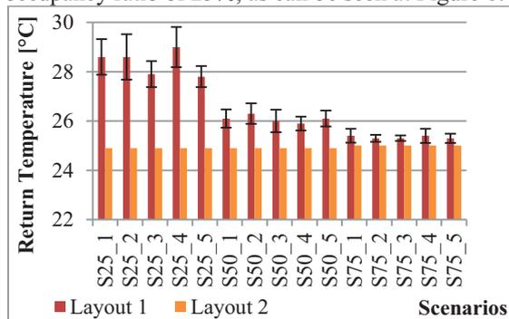
Figure 6. The mean return temperature per each scenario with standard deviation of them, obtained at the heat source
