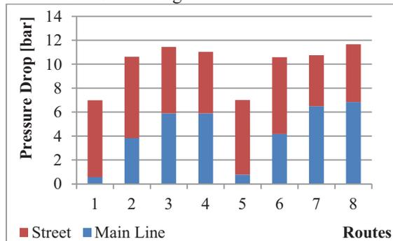
Figure 5. Pressure drop, obtained in main and street lines through the routes
